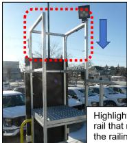
Highlighted in red is the portion of the rail that required collapsing/sliding into the railing tubing below to fit flush with the traffic advisor signal sign for clearance height areas.
