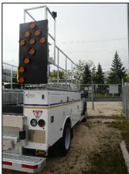
Arrow board incorporated mounting on frame of catwalk
